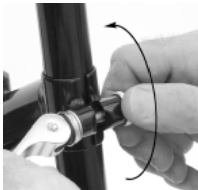
Figure 5c. Adjusting the QR tension.
